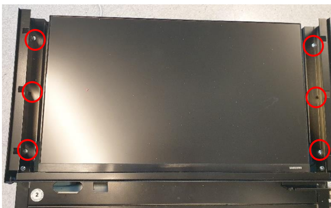
Display frame and its mounting bolts.
