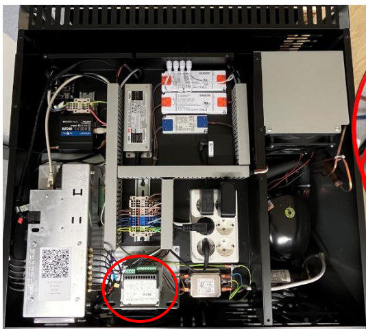
Selfly Model 3 Freezer: Refrigeration system control module location, connectors (1) and mounting clips (2).
