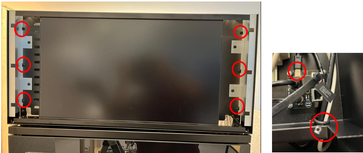
Display frame screw locations and location of universal door cable on component tray.
